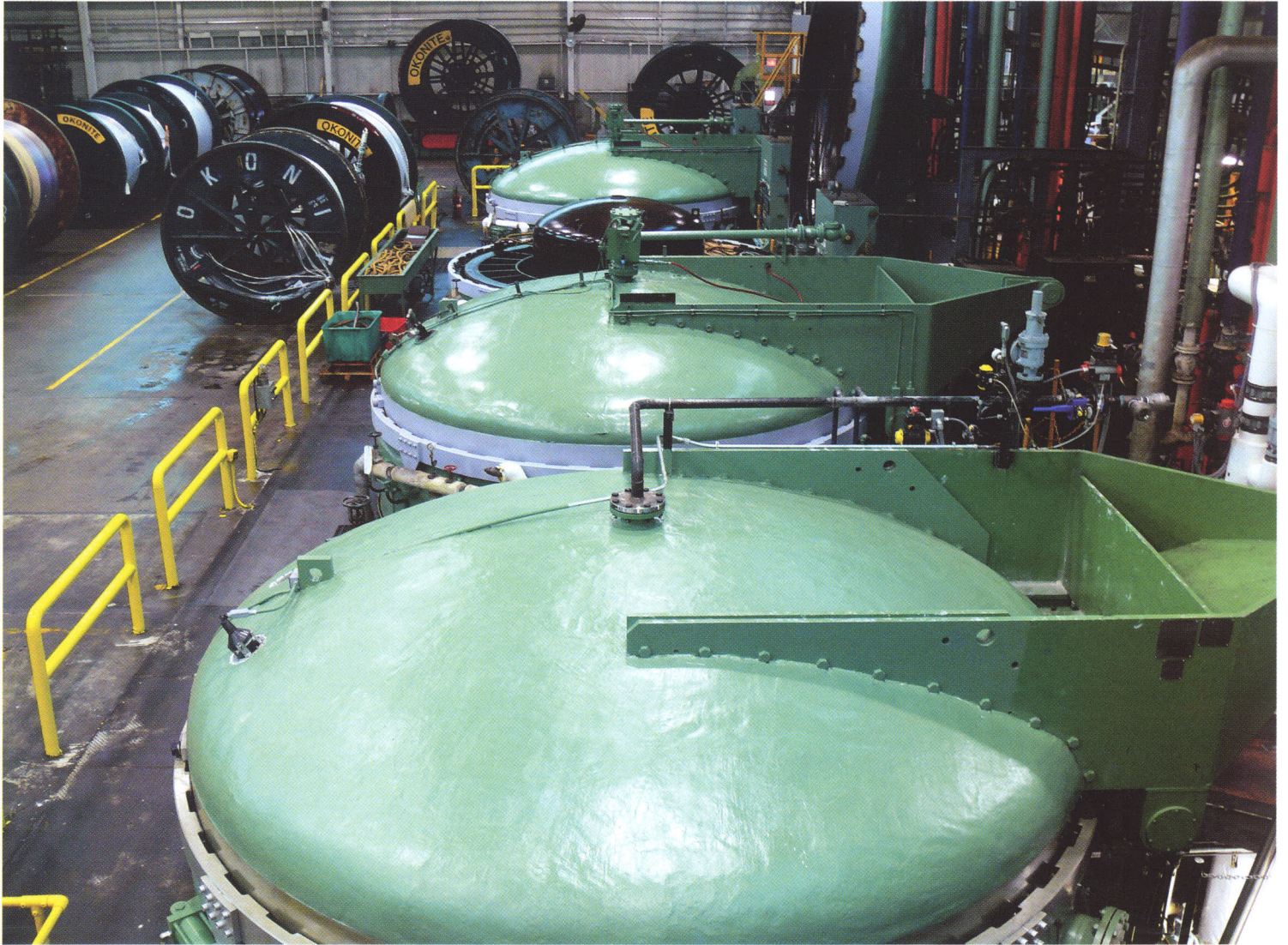
Four Vertical tanks (above and below left) for impregnating up to 345 kv HPFF cables in Lengths of 8,000 to 10,000 feet on 174" diameter reels.
